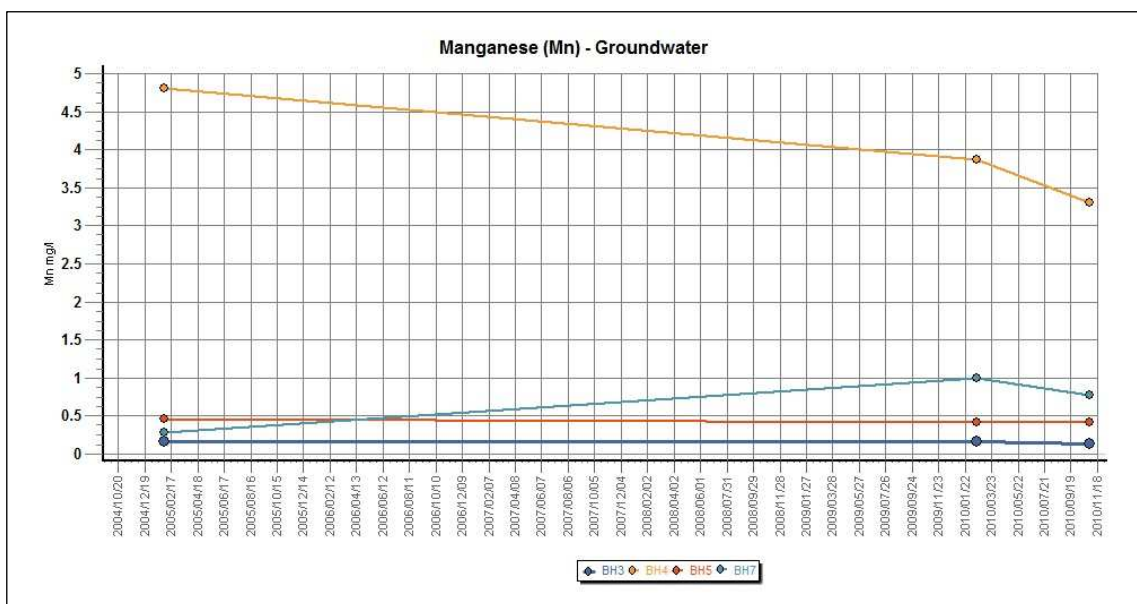
Figure 13: Manganese (Mn) in Groundwater
